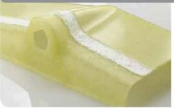
Due to the excellent material properties created by reinforcing the three-dimensionally meshed duroplastic material with glass fibres, GRP has been used for decades to make high-performance products that are expected to have a long service life in tough environments and at the same time ensure high levels of safety. GRP combines the positive properties of steel and plastic.
