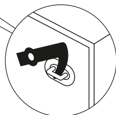
Hooks for securing sides of the container
